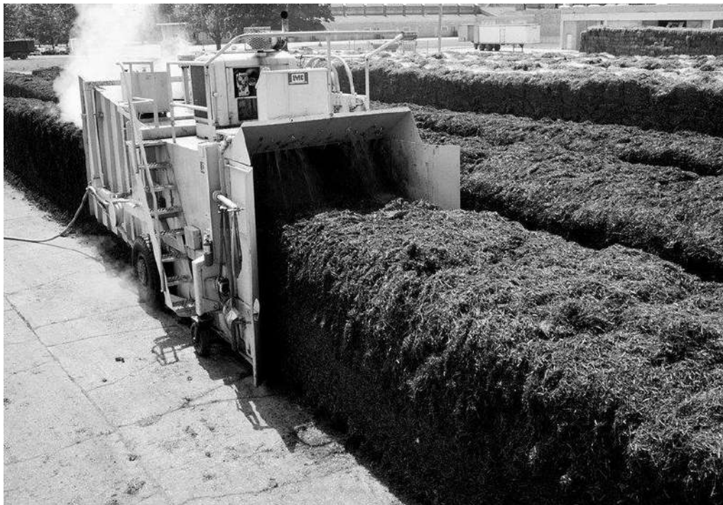
Figure 3 A self - propelled compost piles that moves on top of the compost pile (Royse and Beeline, 2007)
