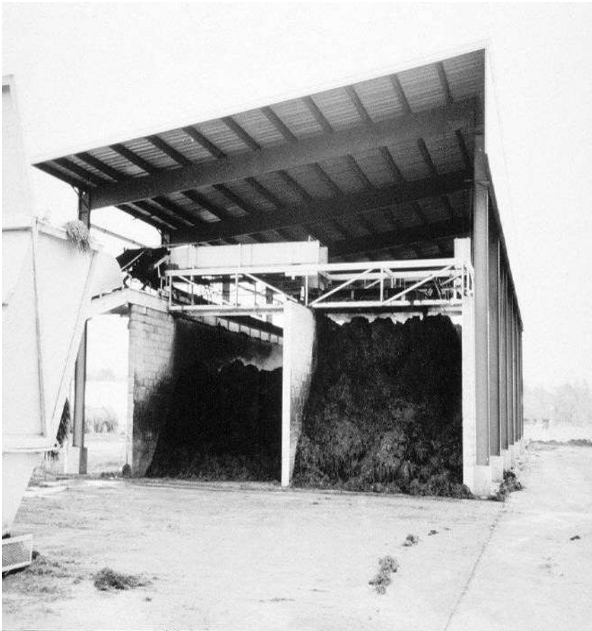
Figure 4 This aerated substrate training device has a piped concrete ground beneath the substrate that forces air through the substrate to hold cardio situations at some point of the composting process (Loehr M.Stephania, 2010)
